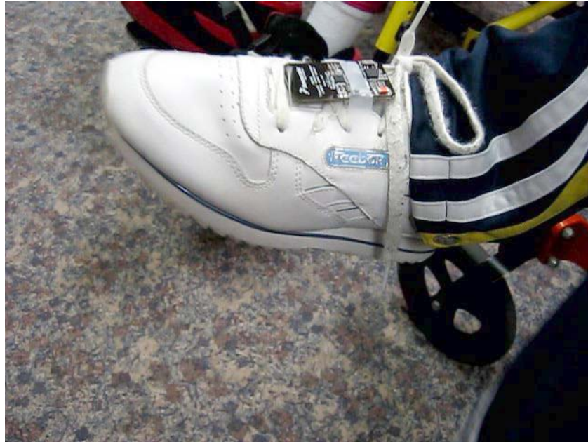
Figure 3: Accelerometer mounted on KJ's athletic shoe.
